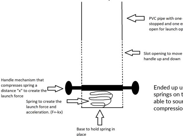
Ended up using two extensions springs on the side due not being able to source the right compression spring
