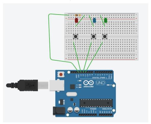
The resistor is placed on the cathode side of the LEDs as to keep the circuit simple and manageable.
