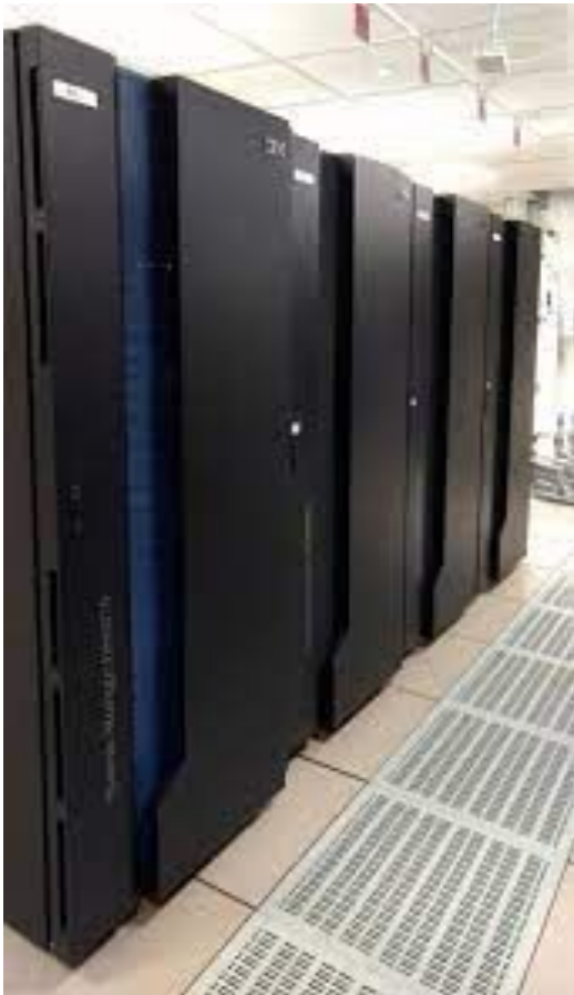
DS8800 storage cabinet
